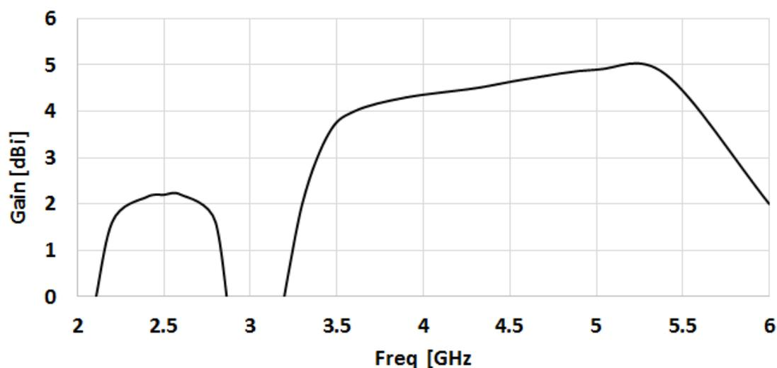
Figure 7. Simulated average gain of the proposed dual band monopole antenna
