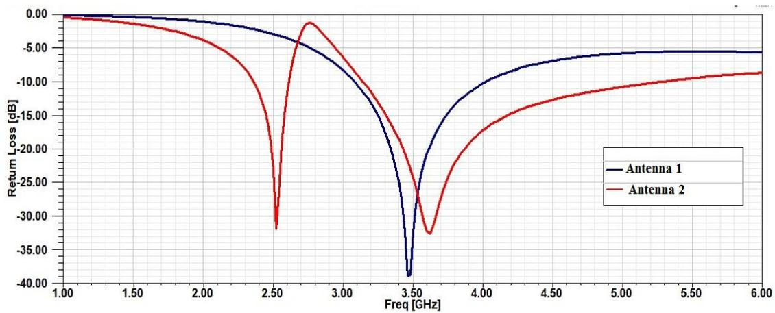
Figure 3: Simulated return loss of antenna evaluation step
