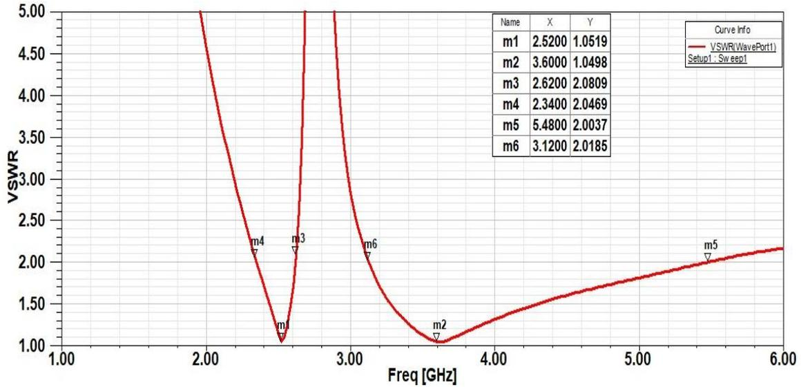
Figure 5: Simulated VSWR of proposed dual band monopole antenna
